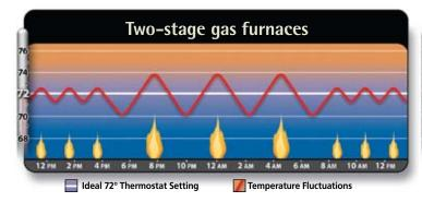
Two-stage gas furnaces offer an intermediate level of performance. Operation varies between first and second stage based on demand. However, indoor temperature levels still fluctuate, relative to your thermostat setting.
